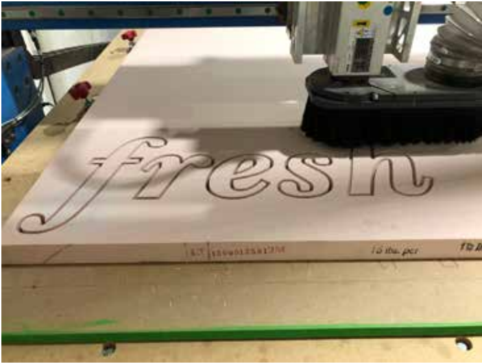
Programed CNC with VCarve to Cut Letters out of HDU Foam Board
